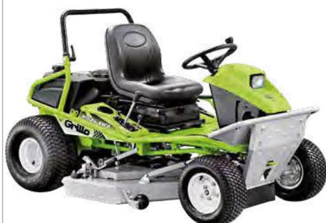
TRANSMISSION 4WD PERMANENTES AVEC EMBAYAGE ELECTROMAGNETIQUE, BLOCAGE DIFFERENTIEL, ARCEAU DE SECURITE, ROUES GAZON, CROCHET D'ATTELAGE, SIÈGE AVEC SUPPORT AMORTI
