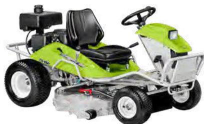
EMBAYAGE ELECTROMAGNETIQUE, ROUES GAZON ET CROCHET D'ATTELAGE
